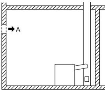
$$A = 150 \text{ см}^2 + 2 \frac{\text{см}^2}{\text{kBt}} \times (\Sigma \dot{Q}_n - 50 \text{ кВт})$$
